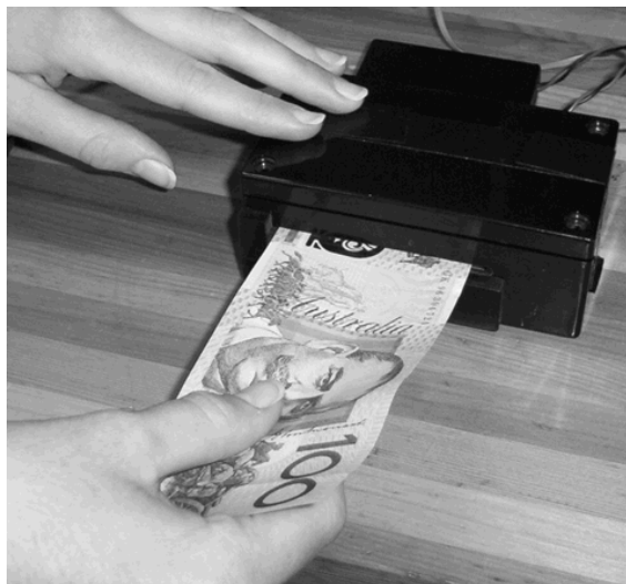
Figure 3. The prototype Money Talker in use. The system is showed connected via a serial line to a PC for the purposes of testing.
